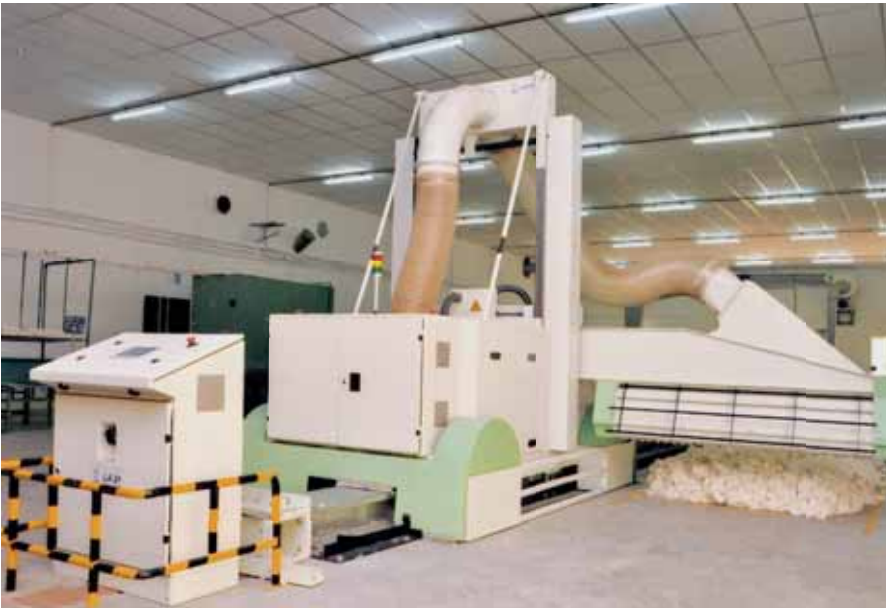
A view of the LMW make Swift Floc Bale Plucker machine in Blow room installed at our Textile Division, Sri Ramco Spinners, Rajapalayam.
