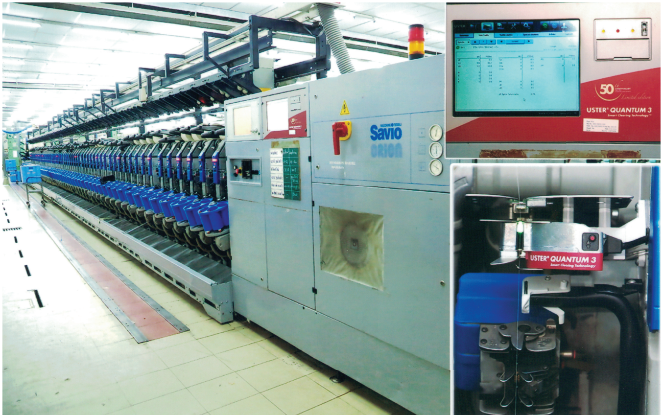
USTER QUANTUM – 3 installed in Automatic Conewinding machine for online control of yarn quality, at our Textile Division, Sri Ramco Spinners, Rajapalayam
