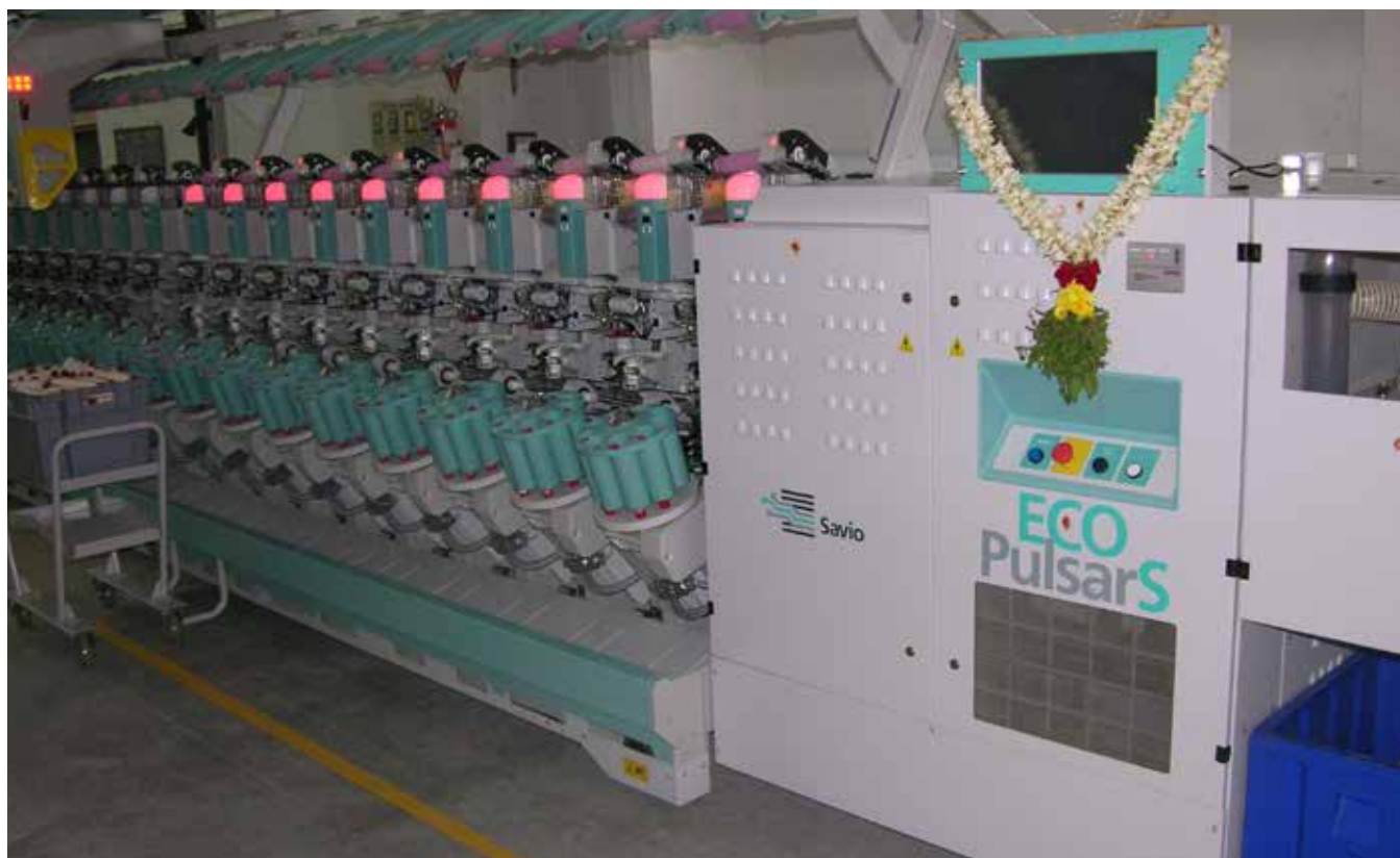
SAVIO ECO PULSARS – L MULTICONE WITH 90 SPINDLES AUTOMATIC CONEWINDER MACHINE INSTALLED AT OUR TEXTILE DIVISION, SRI RAMCO SPINNERS, RAJAPALAYAM
